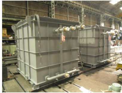
Photograph 2 Seawater Circulation Purifying Facility
